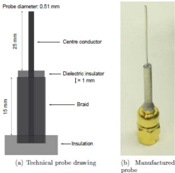
Figure 1. The m-NLP instrument probe [8]
