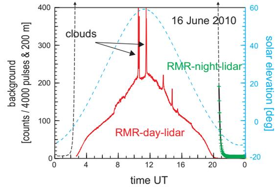
Figure 1. Background variation for the daytime Rayleigh-Mie-Raman (RMR) detector (red) and the nighttime RMR detector (green), 16 June 2010. The dashed black lines show a simulated background for the nighttime detector. At these times no observations are possible because the background increases by many orders of magnitude. The dashed blue line shows the solar elevation.
