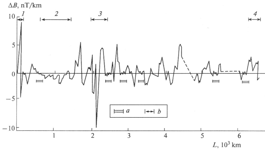
Figure 1. Vertical gradient of the anomaly EMF derived at the altitude  $h = 30$  km. (a) Profile portions where magnetic anomalies are absent; (b) profile portions that divide the territories with the following objects: (1) Klyuchevskaya volcanic group, (2) Sea of Okhotsk. (3) Aldan shield, (4) Kama-Emba magnetic anomaly.
