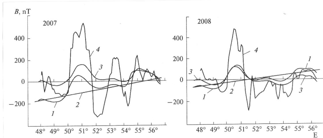
Figure 2. Magnetic anomalies along the stratospheric balloon drift route; (1) distinguished by the IGRF model ( $h = 30$  km); (2) trend connecting portions where magnetic anomalies have no significant values; (3) with the excluded trend ( $h = 30$  km); (4) derived from the map [6] ( $h = 0$ ).
