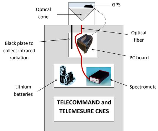
Figure 3: Configuration of the mini SAOZ payload for the first flight
