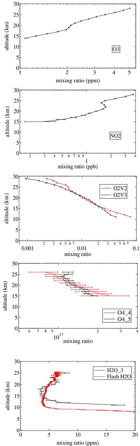
Figure 5: Vertical profiles of species mixing ratio at sunset derived from the first mini-SAOZ flight. From top to bottom: O<sub>3</sub>, NO<sub>2</sub>, O<sub>2</sub>, O<sub>4</sub> and H<sub>2</sub>O.
