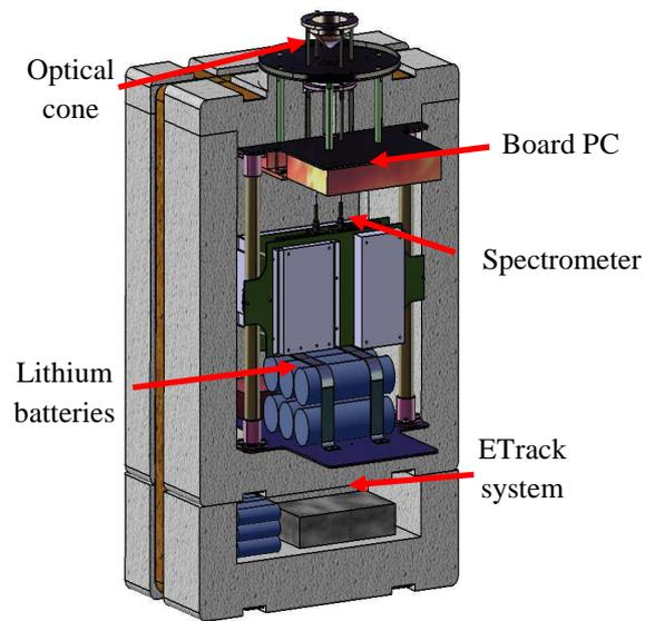
Figure 7: Design of the mini SAOZ payload
