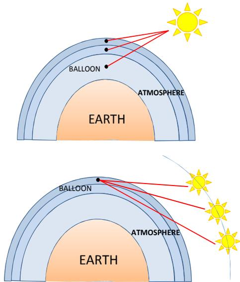
Figure 2: Solar occultation measurements during the ascent at  $SZA < 90^\circ$  (top), and during sunset from float altitude at  $SZA > 90^\circ$  (bottom)
