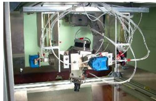
Figure 9. Prototypic realization of Platform Orientation Mechanism (POM) for BEXUS 11 flight
