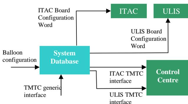
Figure 8: the system database, core of the adaptability of the TMTC interface
