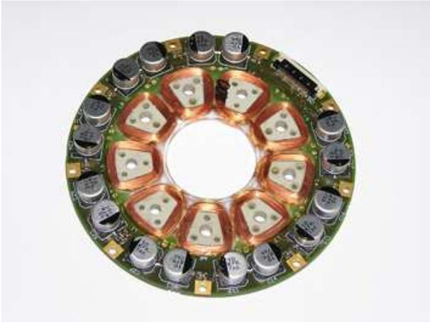
Figure 5. The corner stone of the Digital Direct Drive concept; tight integration of the drive stage with the motor armature on a single hybrid substrate.
