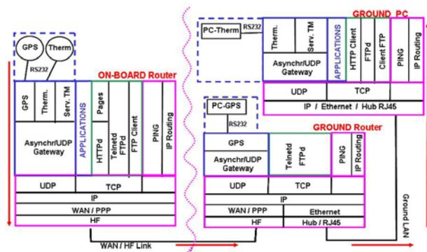
Figure 2. Overview of ETNA 2 TCP/IP architecture
