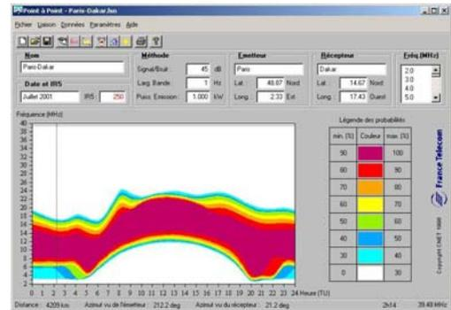
Figure 8. Example of hard copy of the dedicated software used to calculate the exact working frequency
