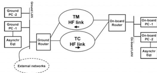
Figure 1. Principles for an IP architecture in the balloon context
