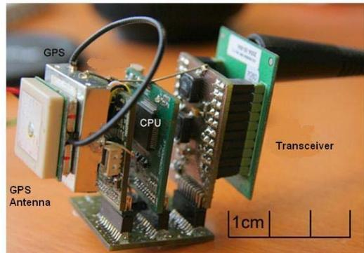
Figure 3. NANO gondola electronic equipment
