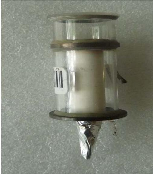
Figure 2. VUV hydrogen glow-discharge lamp
