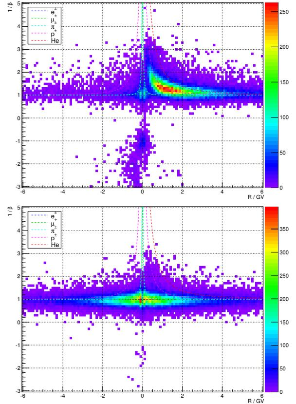
Figure 4. Correlation between reconstructed inverse velocity  $\beta^{-1}$  and reconstructed rigidity  $R$  during float phase (upper) and on ground (lower).
