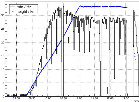
Figure 3. Trigger rate plotted together with the height of the BEXUS-11 balloon.
