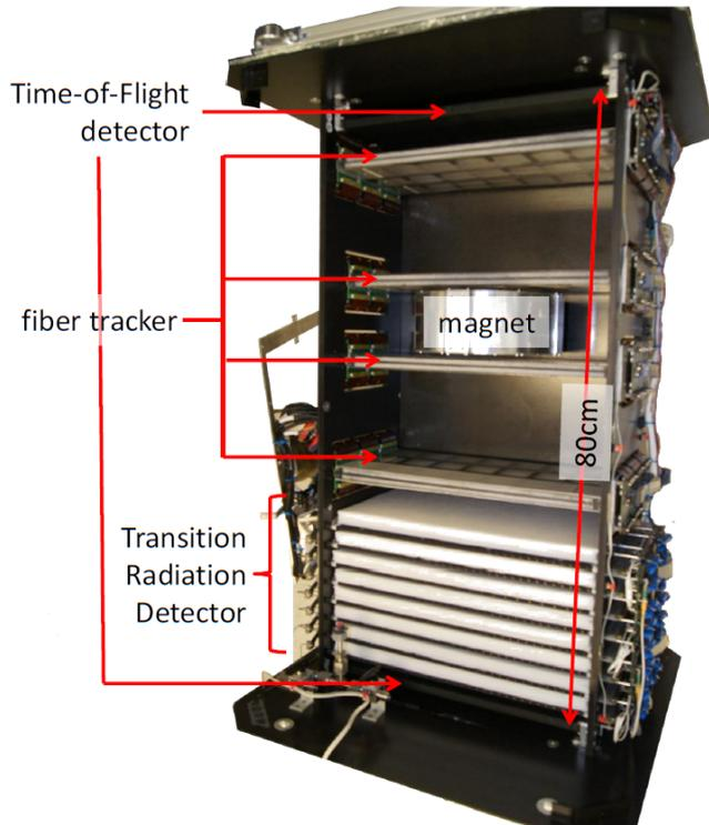
Figure 2. A photograph of the PERDaix detector.
