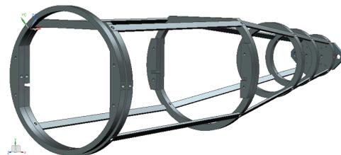
Figure 2. The inner structure of the airframe.
