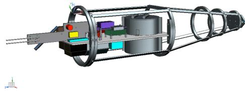
*Figure 3. Placement of the electronics and parachute inside the inner structure.*
