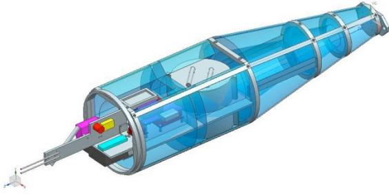
*Figure 4. CAD drawing of the fuselage inner structure. The parachute is housed in the cylinder, located in the centre of the body.*
