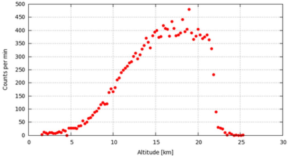
Figure 3. Counts of particles (in counts of CRD detector per minute) as a function of altitude.
