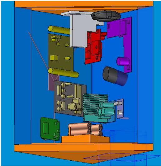
Figure 2. Components of the payload within Julo 1: flight computer (gray), GPS receiver (black at the top), webcam (black in the middle), cosmic ray detector (yellow), accelerometers (purple), battery with electronics (copper, blue), transmitter (green), GSM module (red).
