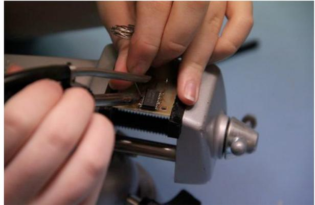
*Figure 4. A student soldering a sensor board*
