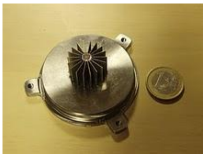
Figure 1. sponge PMD device mounted on its titanium base.
