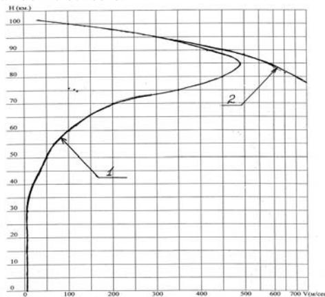
Figure 7. Calculated speed of PS descent
