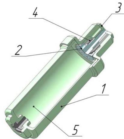
Figure 6. A unit of ethyl acetate vapor injection to a canopy inflation system
