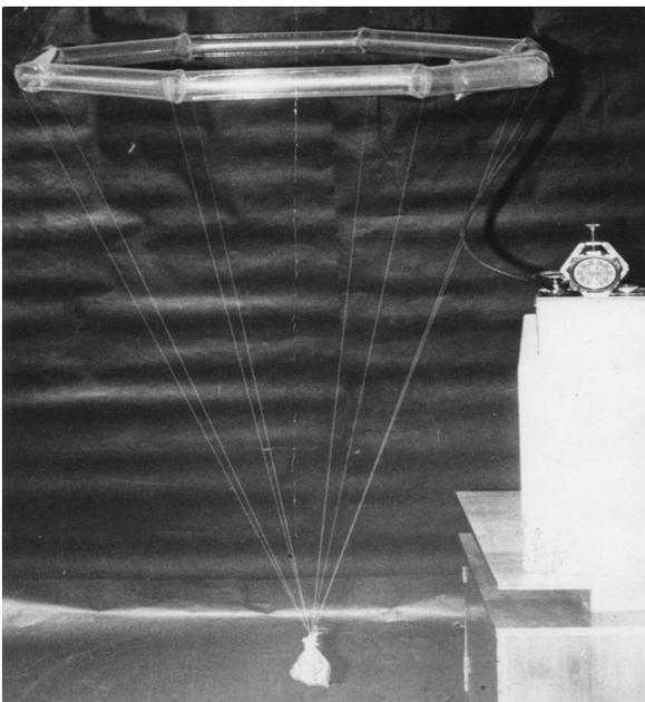
Fig.8. An episode of testing the forced-inflation parachute system.
