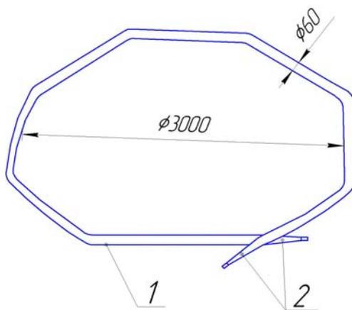
Figure 5. A system of parachute canopy forced inflation
