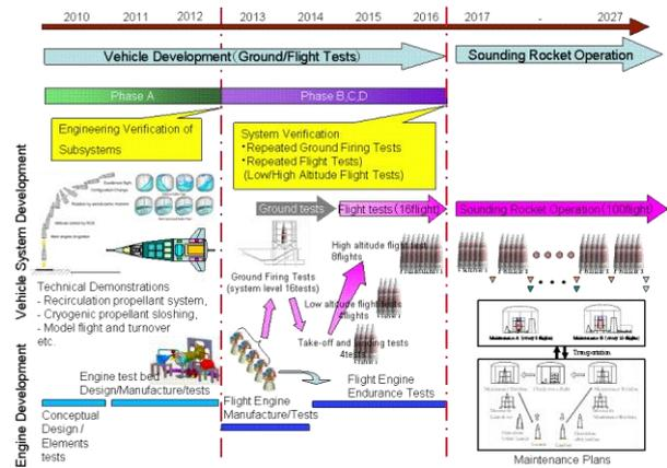
Figure 1. Development plan of reusable sounding rocket.
