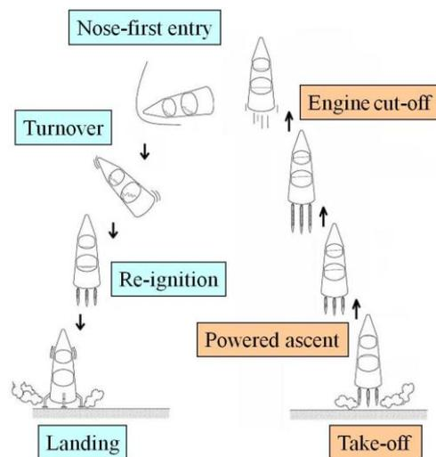
Figure 3. Typical ballistic flight sequence.
