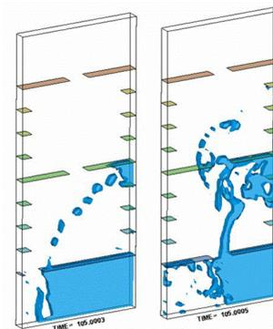
Figure 8. Numerical simulations of liquid propellant sloshing with damping devices.
