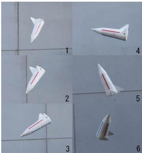
Figure 14. Preliminary glide test for turnover maneuver.
