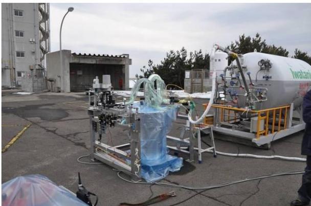
Figure 10. Insulation cycle test by using LH2.
