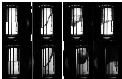
Figure 9. Visualization of LH<sub>2</sub>/LN<sub>2</sub> sloshing.
