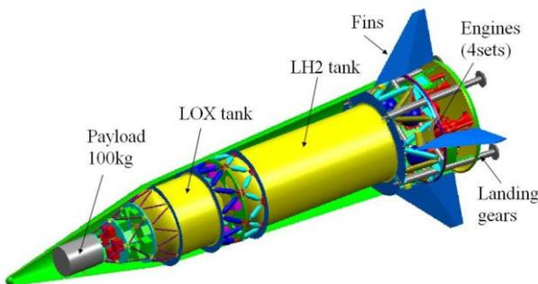
Figure 2. Baseline configuration of vehicle.
