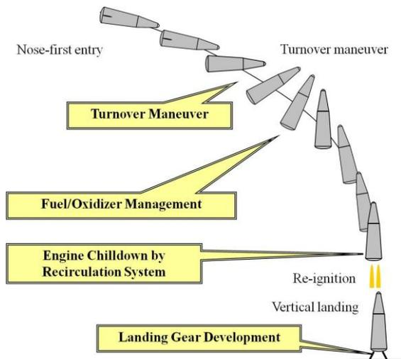
Figure 4. Key technologies in returning flight
