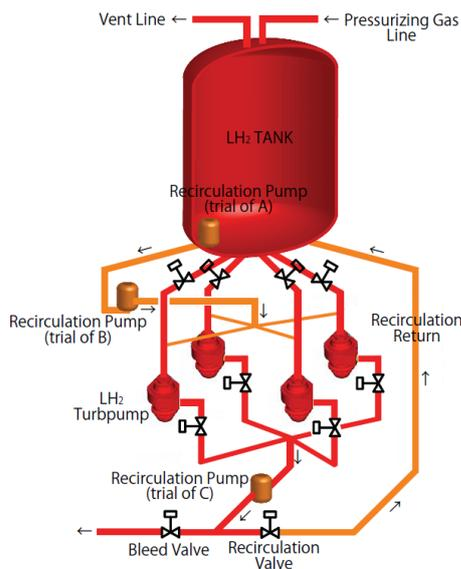
Figure 7. Demonstration of recirculation system.
