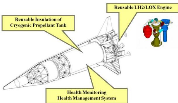
Figure 5. Key technologies in repeated operations.
