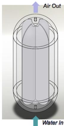
Figure 3. Inner structure (vanes) of the EXPLORE experiment.
