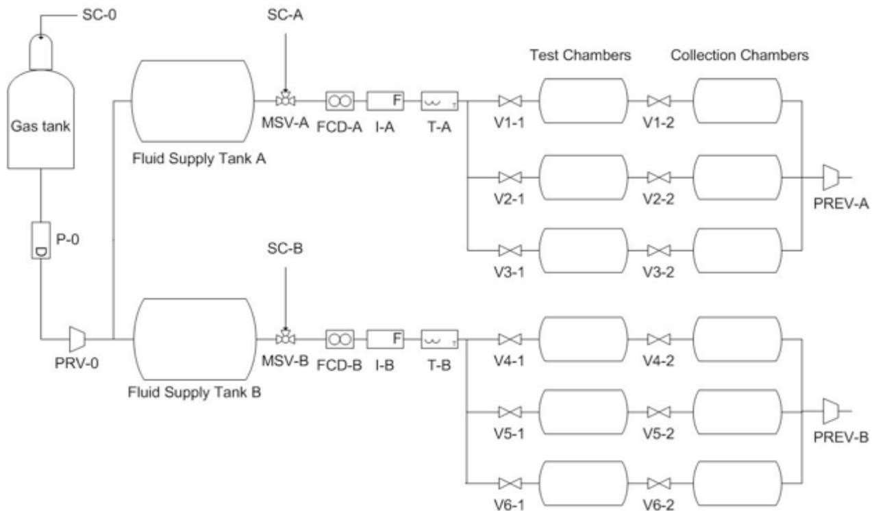
Figure 4. Block diagram of the EXPLORE experiment.
