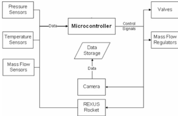
Figure 7. EXPLORE command and data flow.
