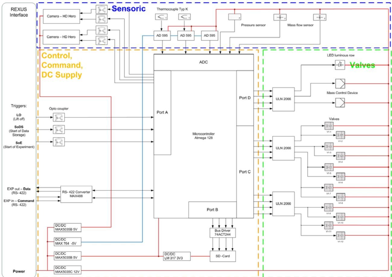
Figure 6. EXPLORE electrical setup schematics.
