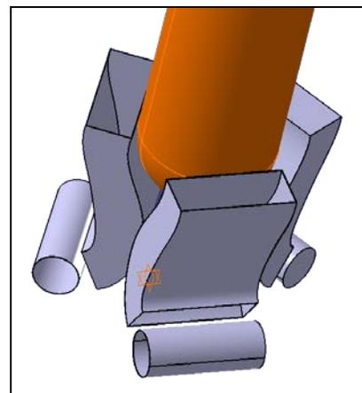
Figure 5. 3D visualization of the three booster configuration with air deflection
