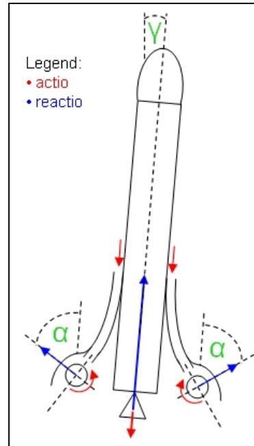
Figure 4. Basic concept of Flettner boosters. Flight angle  $\gamma$  equals ‘0’ for all calculations
