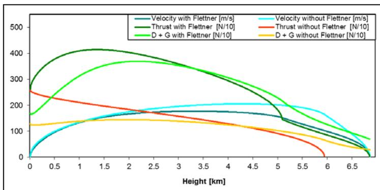
Figure 9. Three booster configuration with 26.3 kg additional payload and 5kg per booster (overall mass of 173 kg). Reached altitude equals 6.86 km (same as baseline with no payload) at a maximum velocity of 177.2 m/s and an ascent time of 64.9 s.
