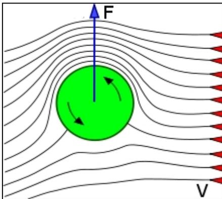
Figure 2. Force  $F$ , resulting from Magnus effect, on a rotating cylinder, held into a streaming fluid Source:Wikipedia
