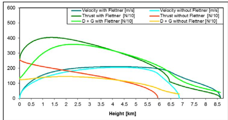
Figure 7. Two booster configuration with 27.3 kg of additional payload and 5 kg per booster (overall mass of 149.7 kg). Reached altitude equals 6.86 km (same as baseline without payload) at a maximum velocity of 183.1 m/s and an ascent time of 64.0 s.
