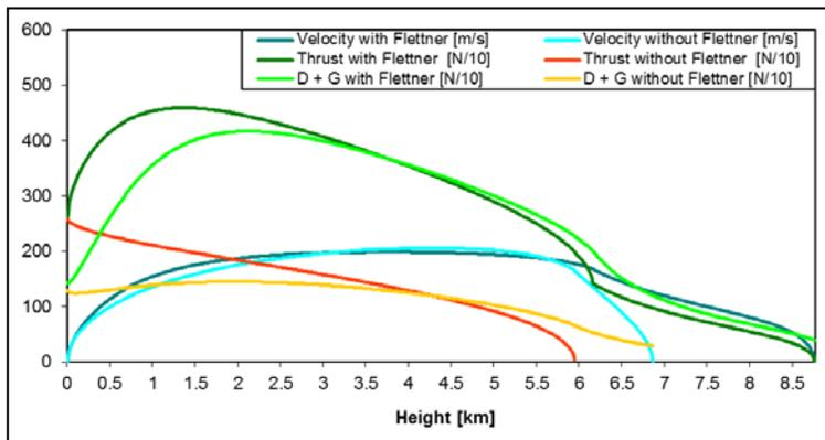
Figure 8. Three booster configuration with no additional payload and 5 kg per booster (overall mass of 146.7 kg). Reached altitude equals 8.76 km at a maximum velocity of 198.5 m/s and an ascent time of 75.8 s.
