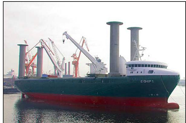
Figure 1. E-Ship 1 with 4 characteristic Flettner rotors on deck, saving up to 40% of fuel Source: Enercon
