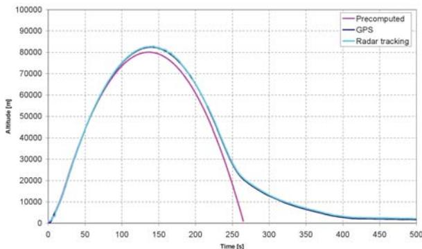
Figure 5. Altitude vs. time plot from Rexus 7 housekeeping data and radar tracking [5]
