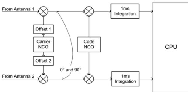
Figure 9. Schematic of the improved system. (N.B.: The in-phase and quadrature signal paths are not drawn separately)
