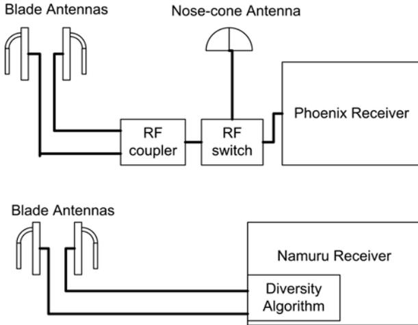
Figure 1. Block Diagram with external components: Phoenix (top); Namuru (bottom)
