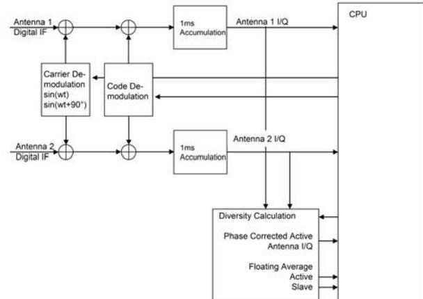
Figure 2. Diversity receiver schematic
