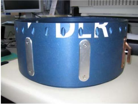
Figure 4. Assembled experiment ring with GPS antenna
