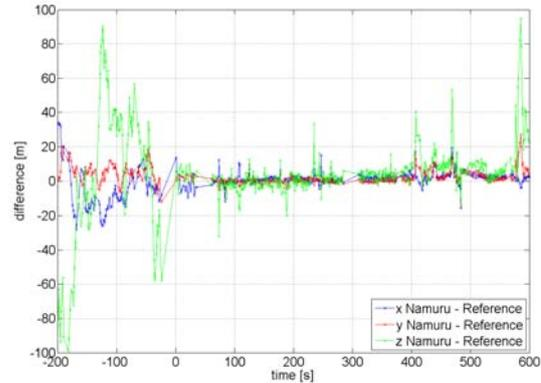
Figure 6. Difference of Namuru-HD and reference receiver
