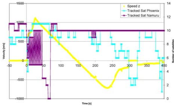
Figure 7. Velocity in vertical direction vs. the number of tracked satellites with Phoenix and Namuru receivers
