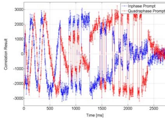
Figure 8. Tracking at 3 Hz in simulation scenario with system flown on Rexus 7
