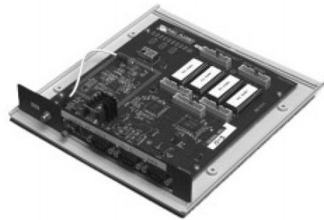
Figure 4 – The GPS Architect main board [6]
