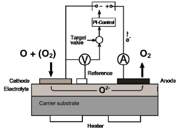
Figure 6: Schematic setup of a 3-electrode sensor.
