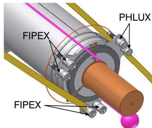
Figure 3: Sensor positions of FIPEX and PHLUX on the upper experiment deck of the sounding rocket.
