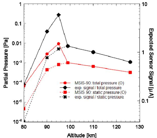
Figure 10: Expected signal for the sensor capable to measure atomic oxygen.
