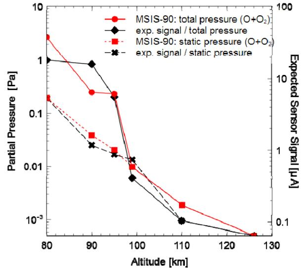
Figure 9: Expected signal for the sensor capable to measure molecular and atomic oxygen.
