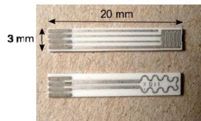
Figure 7: Picture of the screen-printed multi-layer oxygen sensor.
