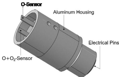
Figure 8: Setup of the sensor head, comprising one sensor for atomic oxygen and one for both atomic and molecular oxygen measurement.
