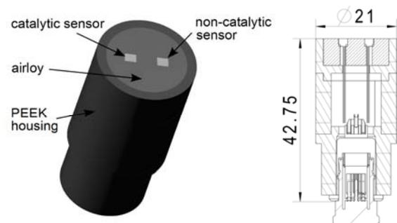
Figure 12: Design of PHLUX sensor head.
