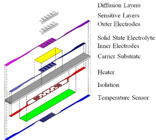
Figure 5: Principle design of multi-layer sensor elements manufactured by screen printing and subsequent sintering.
