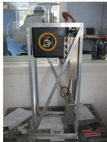
*Figure 3 MAESTRO (in the black enclosure) mounted on the structure used to support it on the gondola. (Post-flight photo courtesy of CNES).*
