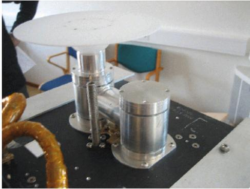
*Figure 2 The MAESTRO omnidirectional light collector. The horizontal tube carries light from the beamsplitter under the collector to the UV spectrometer. (Photo courtesy CNES.)*
