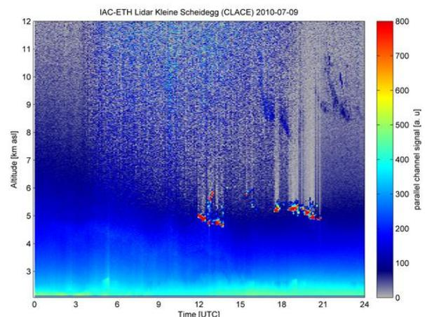
Figure 5. Example of the lidar measurements (parallel channel) showing Saharan dust starting at an altitude of approximately 4.5 km.
