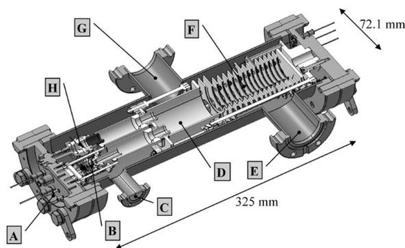
*Figure 1. Engineering drawing of the mass spectrometer. A) Flange with ion source and detector and corresponding electrical feed-throughs, B) ion source with acceleration electrodes, C) sampling gas inlet, D) drift region, E) flange for external turbo-pump, F) ion reflectron region, G) flange for ion getter pump, H) ion detector.*
