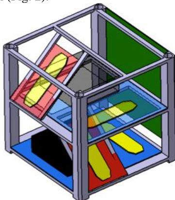
Figure 4. 3D model of a mechanical frame with two redundant electronic boards (green), each having two earth sensors (red) placed with a 90 deg. offset. The offset is necessary to make sure that two axis are measured and that the sensor will be able to point to the Earth at all times.
