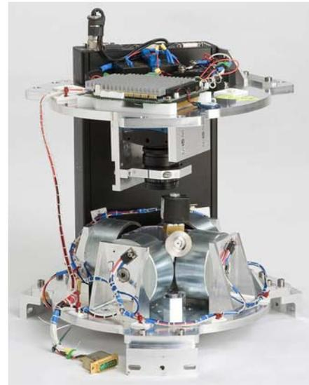
Figure 4: MEGRAMA setup of MAPHEUS 2. A camera records the movement of a granular gas. Credit: DLR-MP
