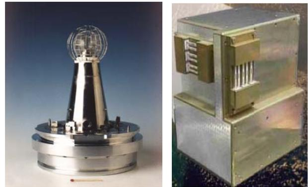
Figure 1: Left: CONE - Combined Sensor for Neutrals and Electrons. Right: FIPEX atomic oxygen sensor flown on the ISS.
