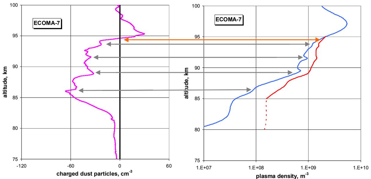
Figure 4 Naturally charged dust collected by the ECOMA instrument in flight 7; the negative sign indicates negative charges (left panel). Electron and ion densities measured in the same flight (right panel). Note the minima of the charged particles coinciding with corresponding maxima in the electron density.
