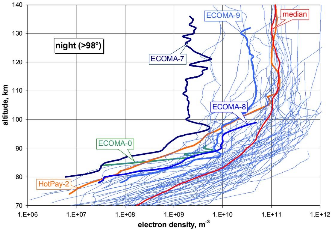
Figure 3 Summary of night-time electron density measurements at high latitudes. The flights referred to in the present context are indicated (primarily ECOMA-7 to -9). Note that these flights are all below the median and furthermore that ECOMA-7 shows the lowest electron densities ever measured.
