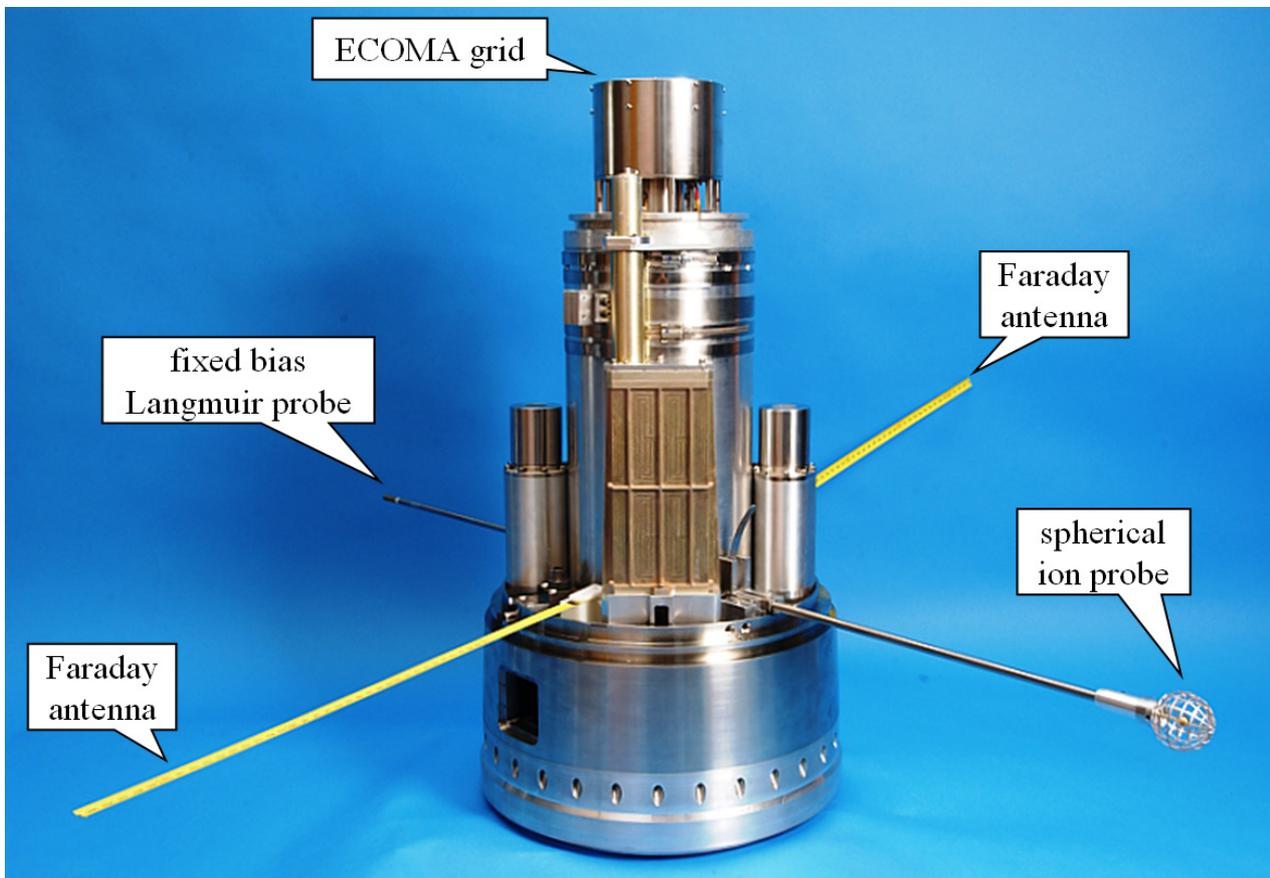
Figure 2 Forward section of an ECOMA payload in flight configuration.
