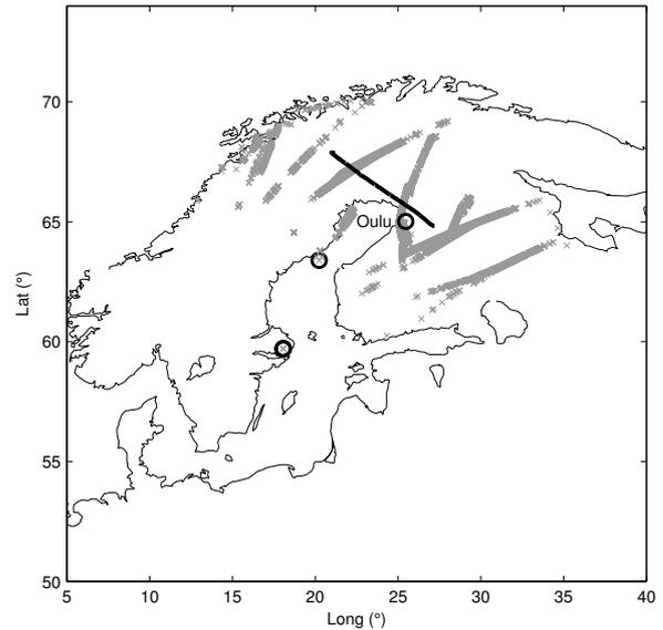
Figure 4. Map of the BEXUS-11 flight. The track of the balloon flight is indicated with a black line. ADS-B position messages are shown in gray x's. Note the aircraft beyond line of sight from the balloon at 50.7 °N, 18.1 °E and at 63.4 °N, 20.2 °E, indicated with black circles.
