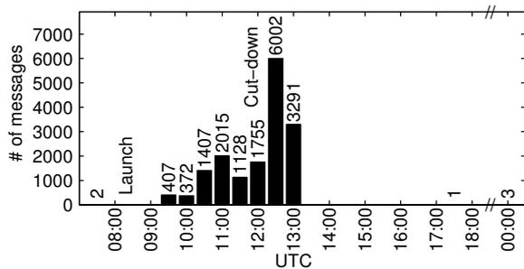
Figure 6. Histogram of the received time of all ADS-B messages for the BEXUS-11 flight
