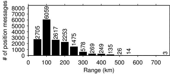
Figure 5. Histogram of the range of all received ADS-B position messages for the BEXUS-11 flight
