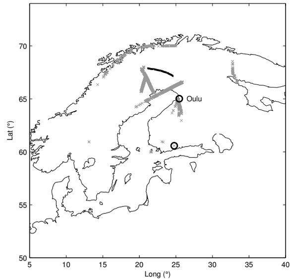
Figure 1. Map of the BEXUS-10 flight. The track of the balloon flight is indicated with a black line. ADS-B position messages are shown in gray x's. Note the aircraft beyond line of sight from the balloon at 60.6 °N, 24.8 °E, indicated with a black circle.
