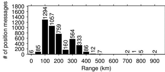
Figure 3. Histogram of the range of position messages received for the BEXUS-10 flight
