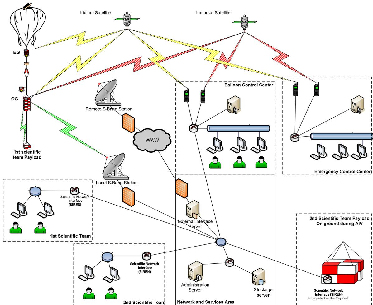
Figure 4. The NOSYCA ground segment
