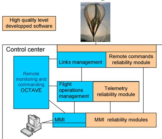
Figure 10. Architecture of CICLOP critical software
