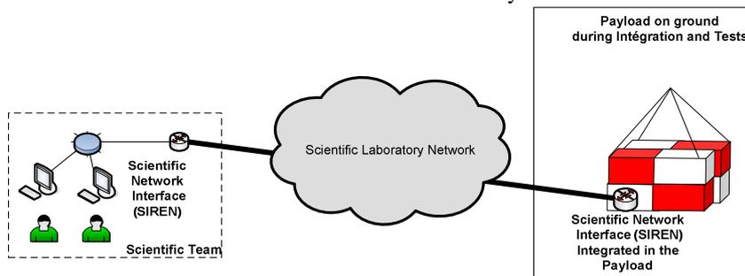
Figure 5. Payload in stand-alone configuration (Note : In bold line the science data transmission)
