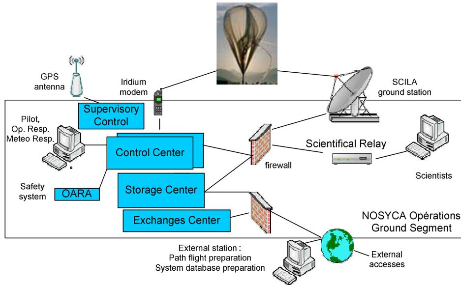
Figure 9. Functional architecture of CICLOP software
