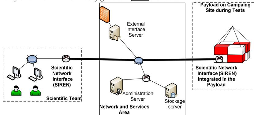
Figure 6. Payload in ground tests on campaign site (payload connected to scientist team through IP NOSYCA ground network)
