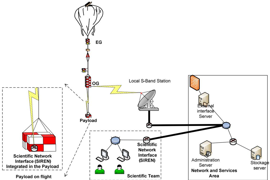
Figure 8. Payload in flight connected to payload control centre through the NOSYCA system
