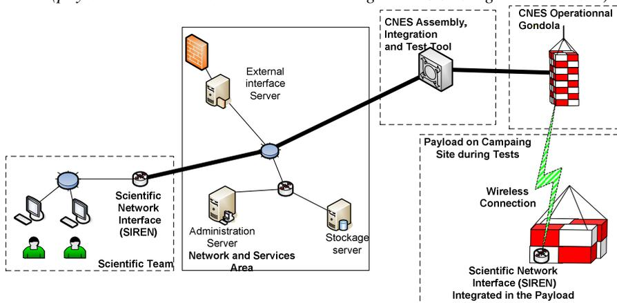
Figure 7. Payload in tests before launch (Payload connected to payload control centre through IP ground network and CNES test bench including the OG)
