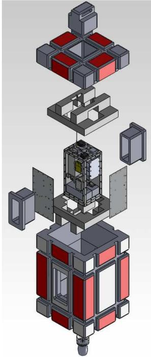
Figure 3. SIRSE module including a RADAR transponder, and a strobe light in the Envelope Gondola
