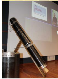
Figure 3. Tank, combustion chamber and nozzle - PEGASE
